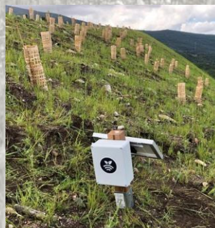
Detail of the humidity sensors placed in the landfill.
