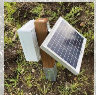
Detail of the humidity sensors placed in the landfill.
